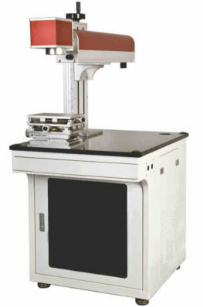
MHX-09-003 Number:MHX-09-003 Product name:Semiconductor cabinet Cabinet Size:740*600*730mm Column Size:170*170*630mm Table Size:150*210mm X=150mmY=90mm
