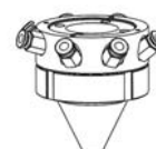
annular powder feeding nozzle
